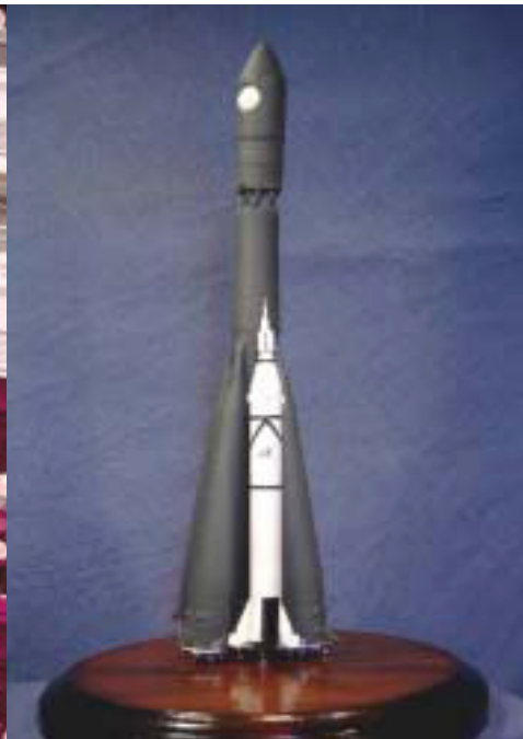
Comparison of the Juno I and R-7 launchers. The R-7 generated ten times more thrust. The models are in 1/144th scale. Models built by Barry Davidoff.
